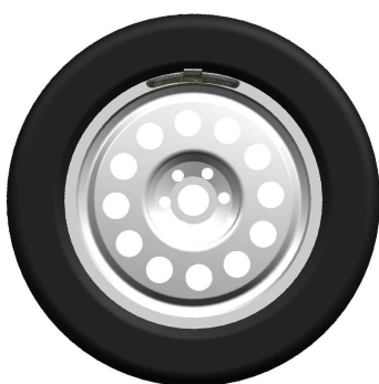
100g WEIGHT TO BE FITTED TO CORRECT UNBALANCE
