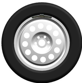
100g WEIGHT TO BE FITTED TO CORRECT UNBALANCE
