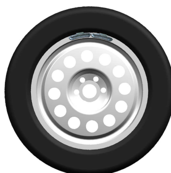
TWO SMALLER WEIGHTS (55g) USING SPLIT PROCEDURE
