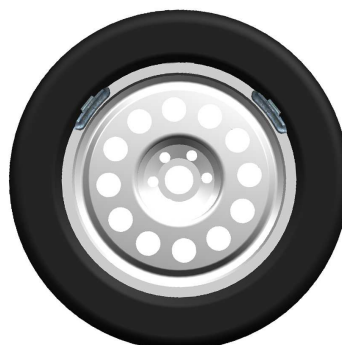
TWO SMALLER WEIGHTS (55g) USING SPLIT PROCEDURE
